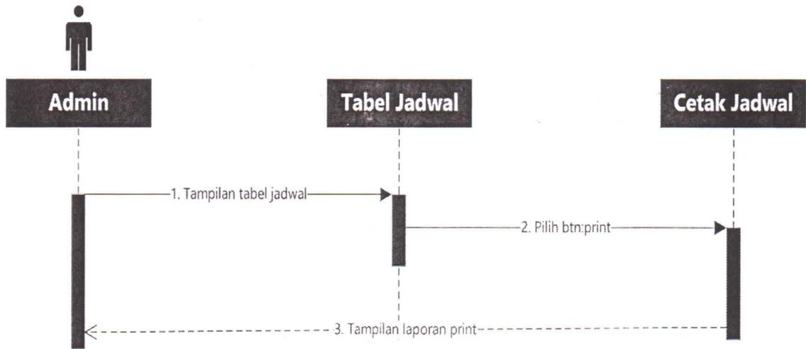
Gambar 4.6 Sequence Diagram Cetak
