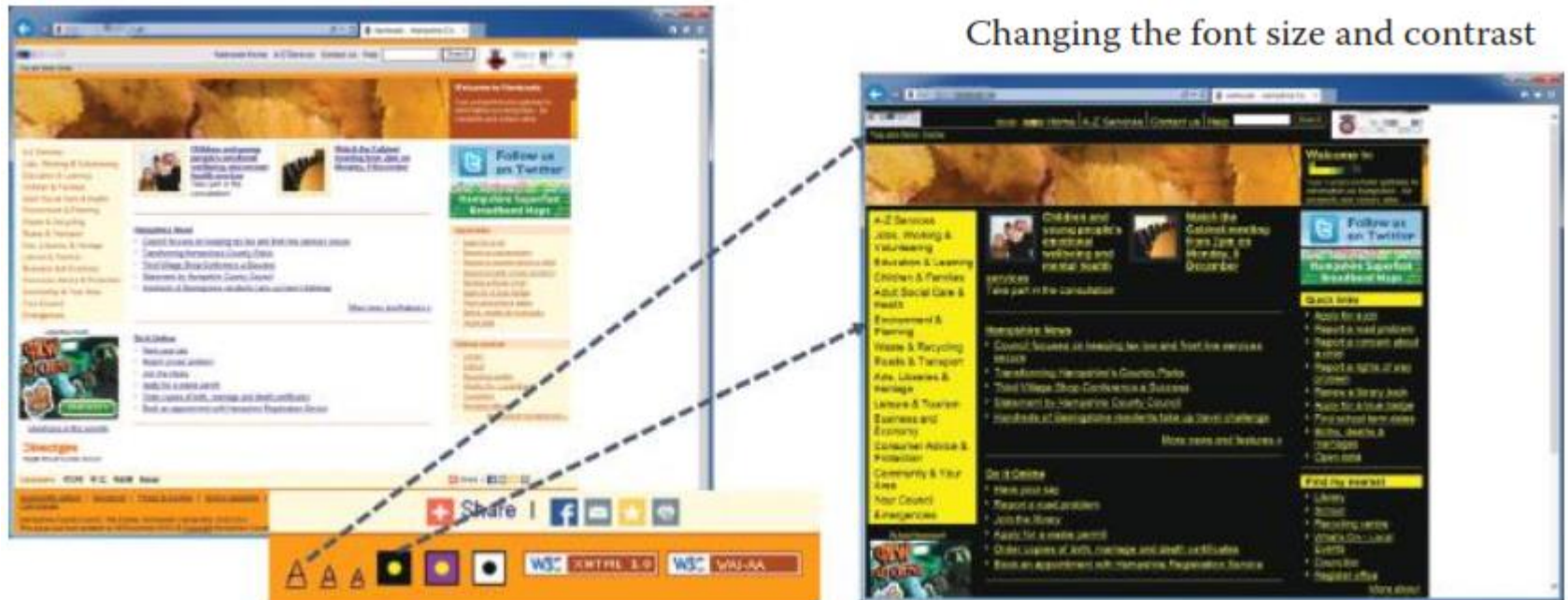
Figure 2.4 Adjustment feature for visually challenged users. The colors of the background and foreground text can be changed.
