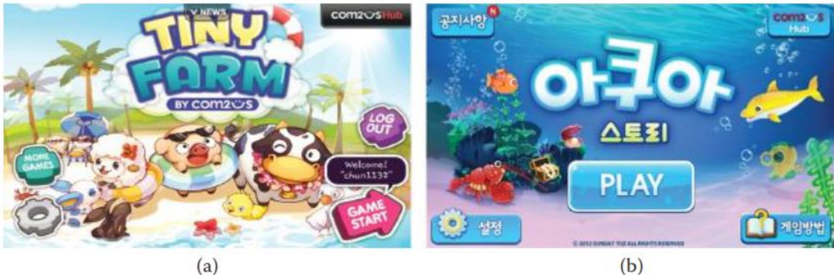
Figure 2.5 Comparison of two mobile game interfaces (the initial entry screen): (a) information and object density is needlessly high and distracting (left), (b) simple and minimal layout, and object sizes fitted to ergonomic usage (right). (From http://www.withhive.com. )
