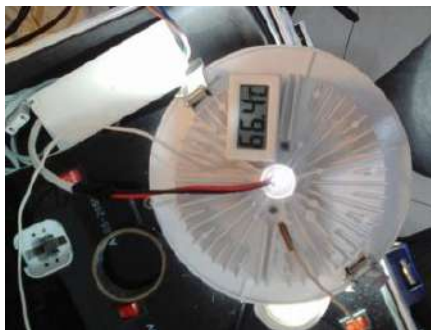
Gambar 1.8 Cacat Over Heat
