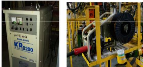
Gambar 6.6 CO 2 Arc Welding
