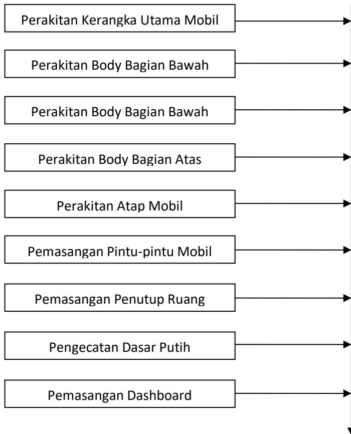
Gambar 6.1 Proses Perakitan Body Mobil di Lini Body Shop
