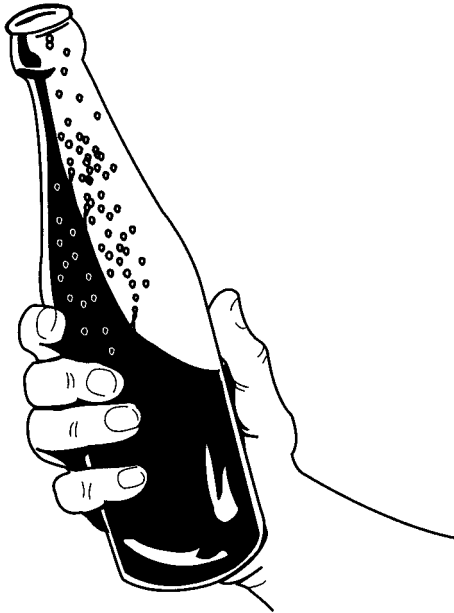
Figure 3-4 The amount of gas dissolved in solution is directly proportional to the pressure of the gas over the solution.
